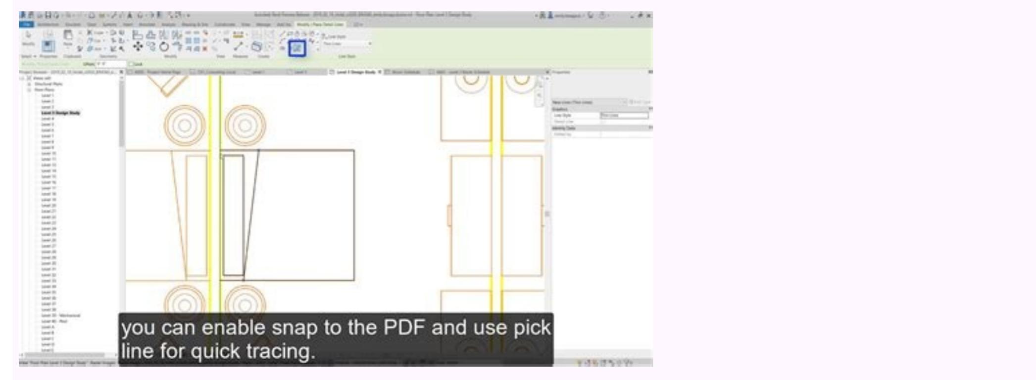
you can enable snap to the PDF and use pick line for quick tracing.
